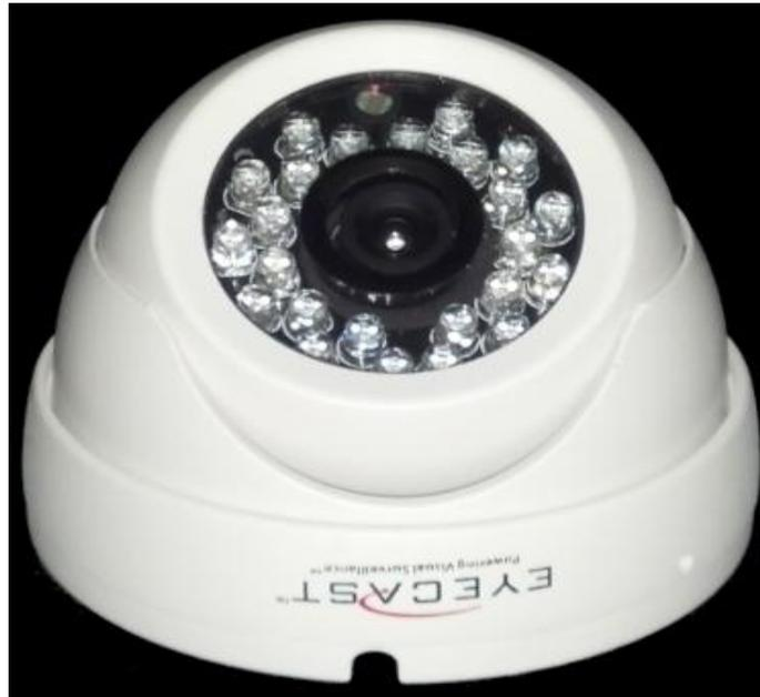
**Description:** IR Vandalproof Dome Camera. High Resolution (700TVL) Digital Color CCD Video Surveillance camera using the latest Sony Effio chipset, 6.0mm lens (slight zoom), true day/night mode for sharp images in both daylight and dark environments. WDR, real time image adjustment, mirror image, sharpness, and eclipse. Easy knob adjustment for focus and zoom.
